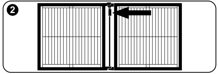
2. Turn hinge locks between each panel counter-clockwise to lock gate in position. Reverse to release. OPTION: For larger animals, leave 2 half-panels operational and use latch at connecting end for opening.
